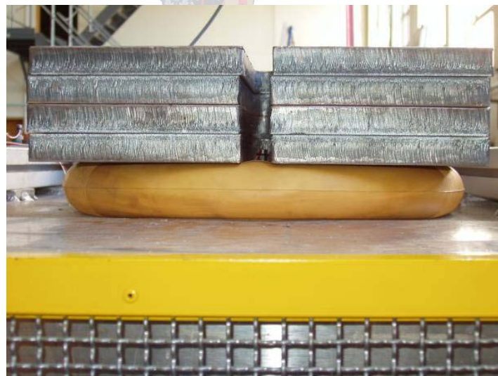
Figure 36 :- 62kg static mass on tube torus during dynamic testing
