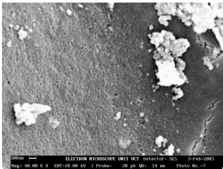
Figure 5-20. SEM image of SDS-stabilised latex particles, 13 months after preparation (1 mm = 100 nm).
