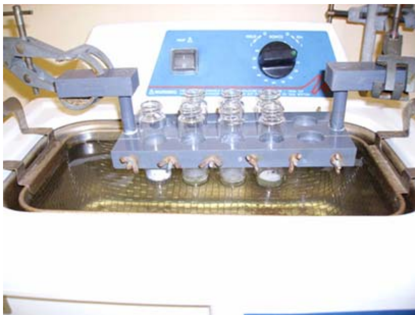
Figure 4.6 Sample holder used during sonication
