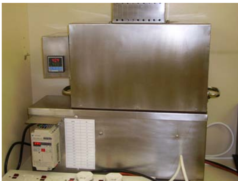
Figure 4.8-B Magnetic stirrer with the oven placed on top of the base plate.
