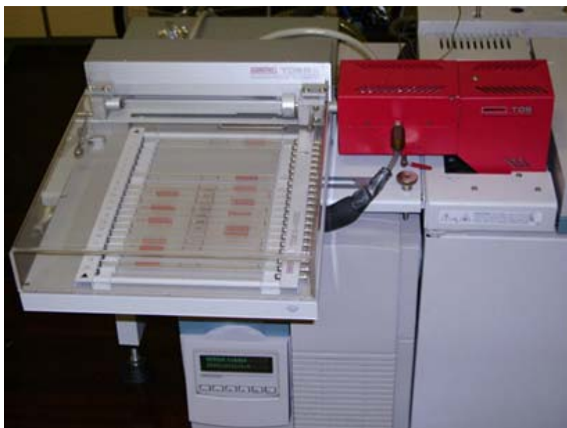
Figure 4.5 The TDS on-line rack
