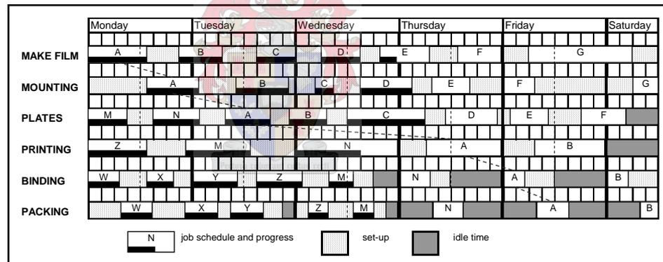
Figure 2.30 : Example of a printing operation schedule
