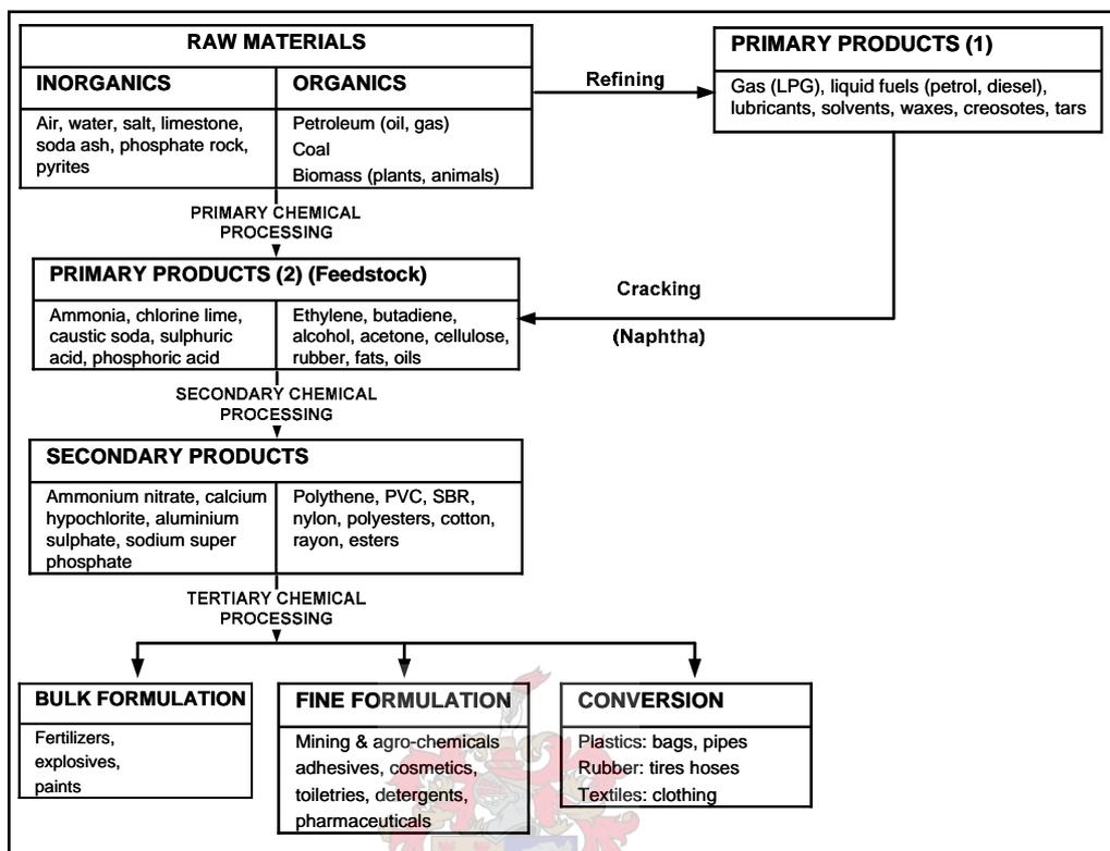
Figure 4.6 : Pipeline model of chemical industry
