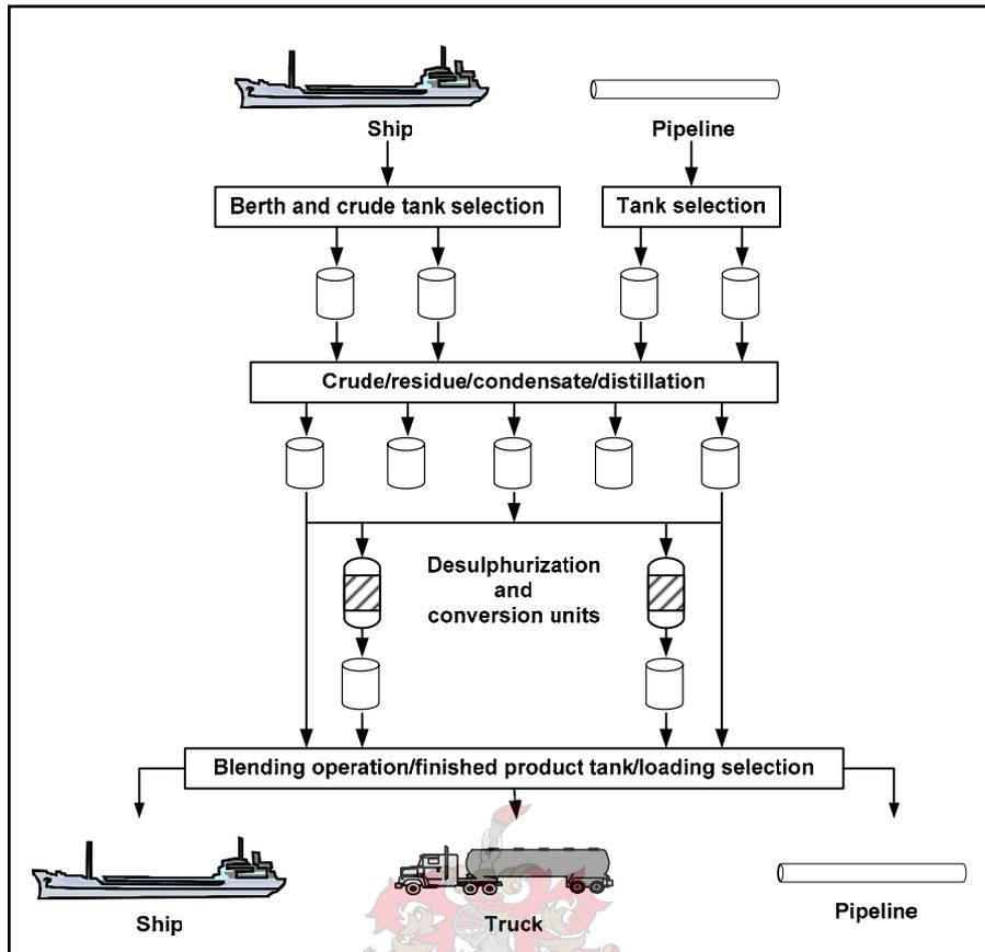
Figure 4.11 : Oil refinery process flow
