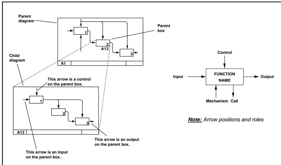
Figure 2.14 : IDEF0 hierarchical series of diagrams
