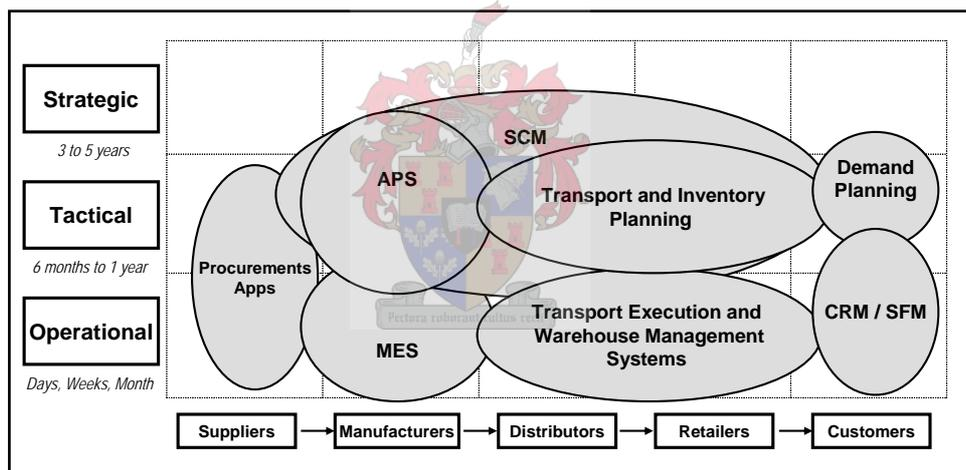
Figure 3.3 : Supply chain IT map – analytical applications.
