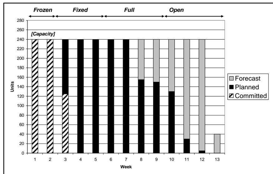
Figure 2.29 : Master production schedule: capacity balanced.
