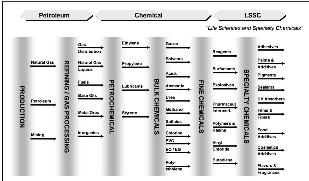
Figure 4.7 : Typical stages in the petrochemicals value chain
