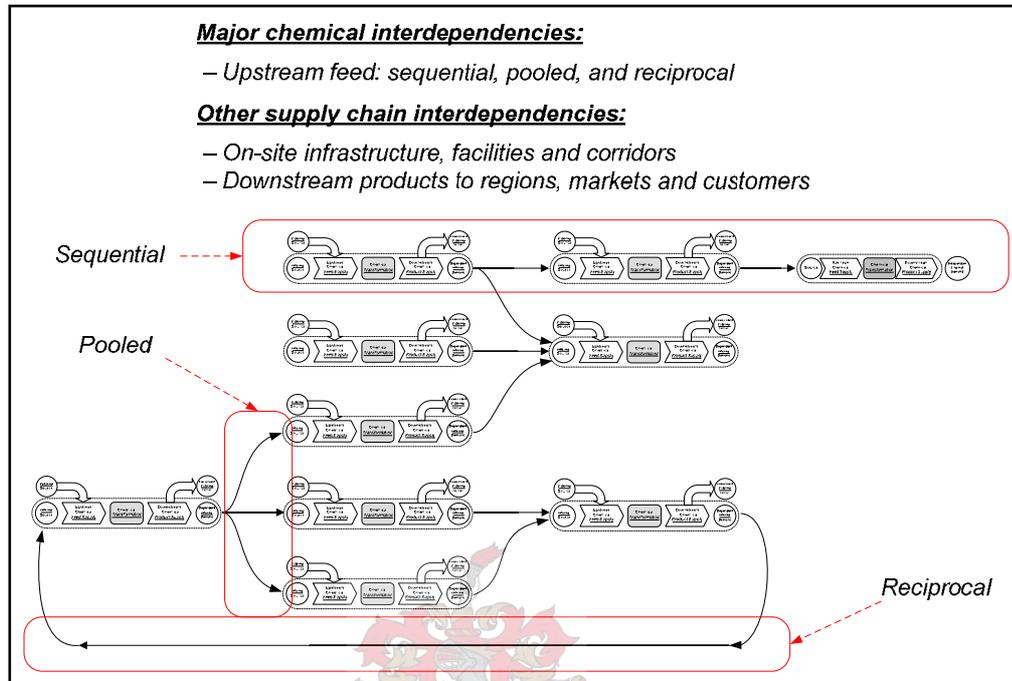
Figure 6.6 : Supply and demand balance (integrated chemical enterprise)
