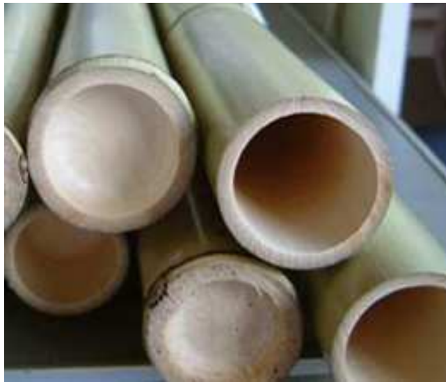
Figure 8-10. Bamboo revealing internal stiffening structures.
