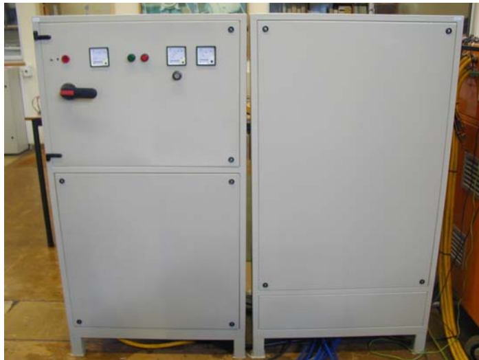
Figure C.2: The complete rectifier and 6-phase full bridge inverter used for the RDCM drive system.
