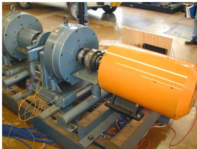
Figure E.3: 6-phase RDCM (orange) and the eddy current dynamometer (blue).
