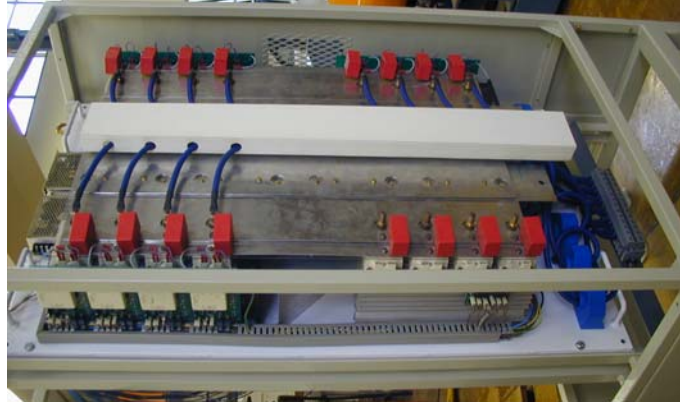
Figure C.1: The 6-phase full bridge inverter showing the SKH121 driver circuitries and DC-bus layout.
