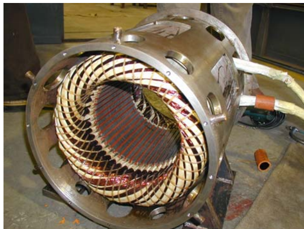
Figure D.3: Stator of the reluctance DC machine.
