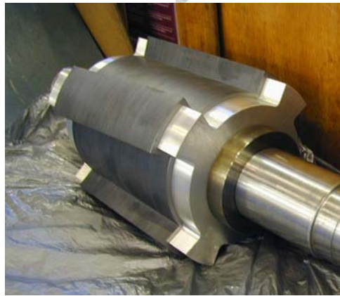
Figure D.2: Skewed rotor of the reluctance DC machine.
