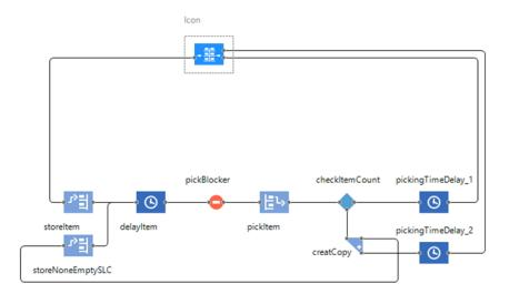
Figure 4-6: Process flowchart of the SLC\_Logic agent
