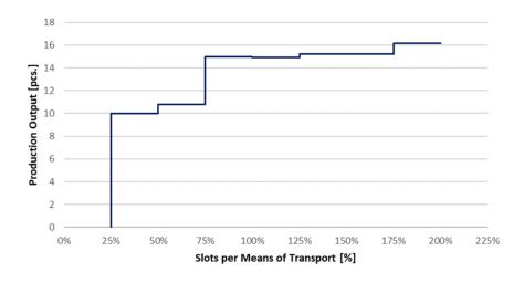
Figure 6-11: Influence of the means of transport capacity on production output
