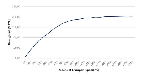
Figure 6-7: Influence of the means of transport speed on throughput
