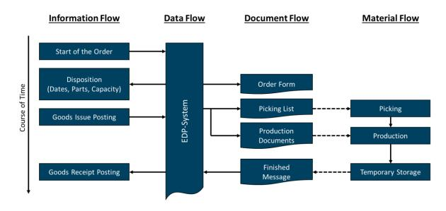
Figure 2-4: Interlinking of information flow and material flow according to Martin (2014, p. 25)
