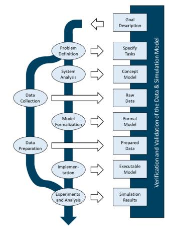
Figure 1-2: Process model of simulation according to Rabe et al. (2008, p. 5)
