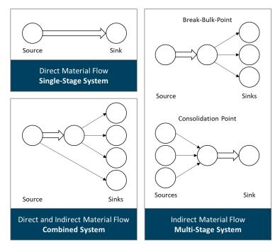
Figure 2-1: Fundamental structures of logistics systems according to Pfohl (2010, p. 6)
