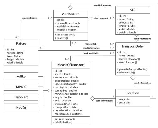
Figure 4-1: Class diagram of Werk150
