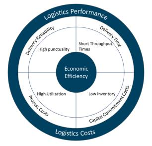
Figure 2-5: Target system of production logistics according to Wiendahl (2019, p. 247)
