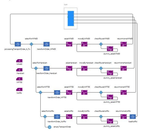
Figure 4-7: Process flowchart of the Transporter\_Logic agent
