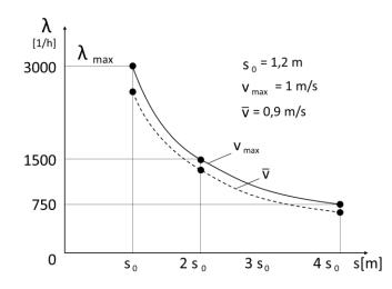
Figure 3-1: Correlation of throughput and distance on a material flow route according to Arnold and Furmans (2005, p. 12)
