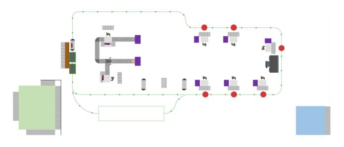
Figure 2-17: Layout of the Werk150 city scooter production
