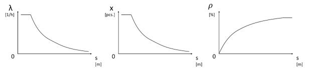
Figure 3-3: Expected behaviour of the material flow route length
