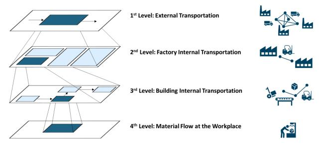
Figure 2-6: Hierarchical levels of material flows according to Bullinger and Lung (1994, p. 5)
