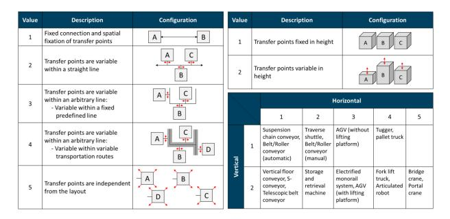
Figure 2-13: Criteria for evaluating layout flexibility according to Heinecker (2006, pp. 74–76)
