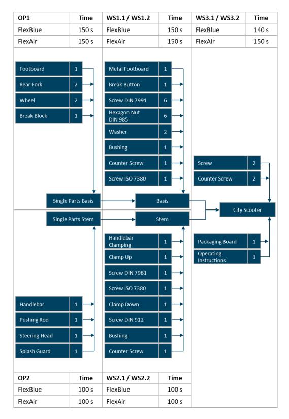
Figure 2-18: Assembly plan of the two city scooters according to Große Erdmann (2020, p. 37)
