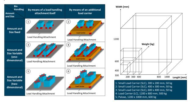
*Figure 2-15: Criteria for evaluating product flexibility according to Heinecker (2006, pp. 81–82)*
