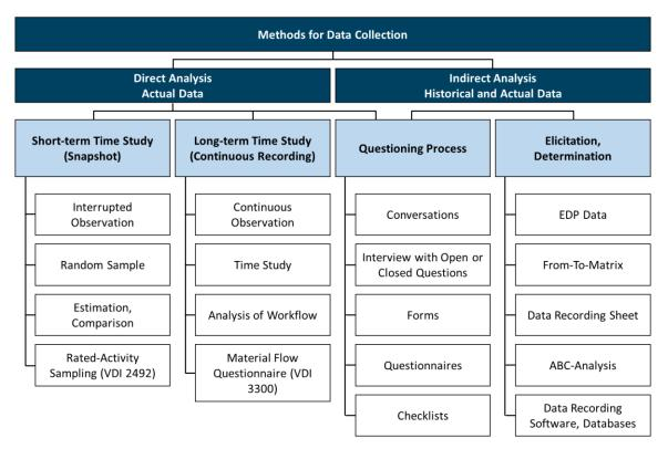
Figure 2-8: Methods for directly and indirectly gathering data according to Martin (2014, p. 464)
