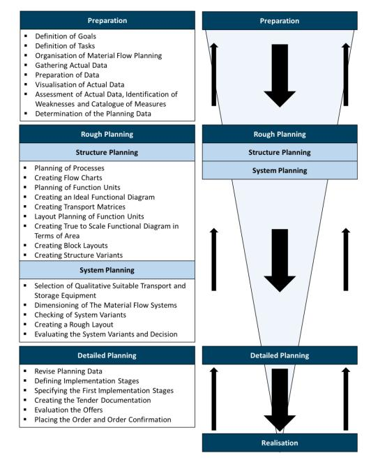
Figure 2-7: Planning approach for material flow systems by Allgayer (1999, p. 26)
