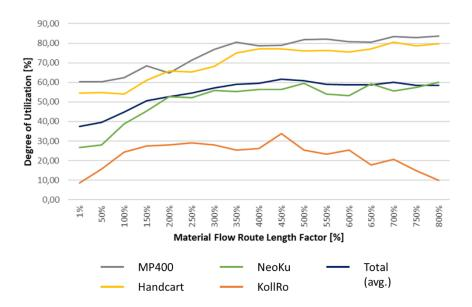
*Figure 6-6: Influence of the material flow route on the degree of utilisation of the means of transport*
