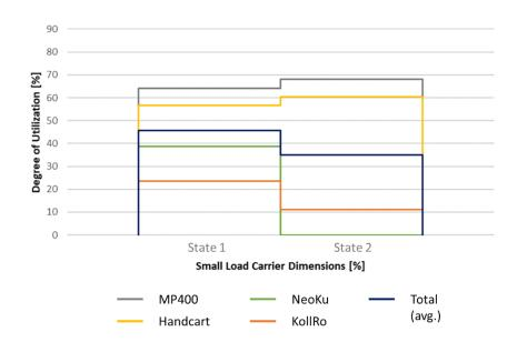
Figure 6-15: Influence of the product dimensions on the degree of utilisation of the means of transport
