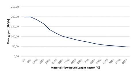
Figure 6-4: Influence of the material flow route on throughput
