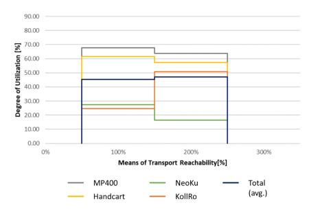
Figure 6-3: Influence of reachability on the degree of utilisation of the means of transport
