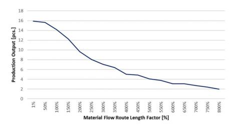
Figure 6-5: Influence of the material flow route on production output
