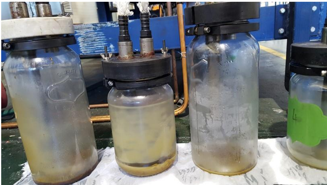
Figure 5.40: Typical distribution of LDPE/PET multi-layer derived oil/wax in pilot scale condensers 1 to 4 (as shown from left to right)
