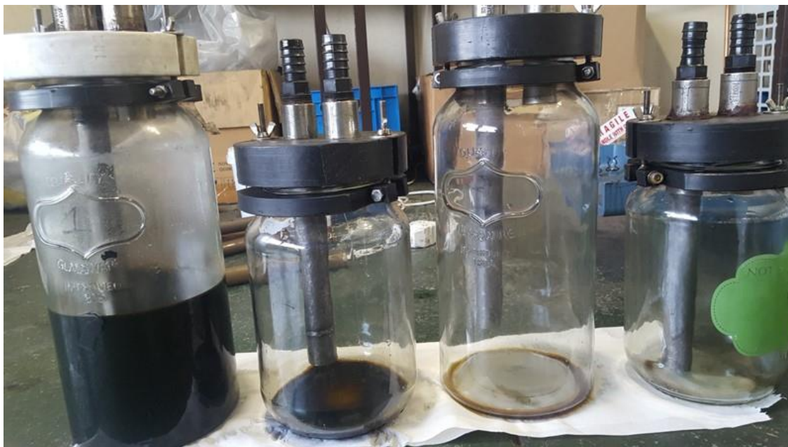
Figure 5.34: Typical distribution of PS derived oil in pilot scale condensers 1 to 4 (as shown from left to right)
