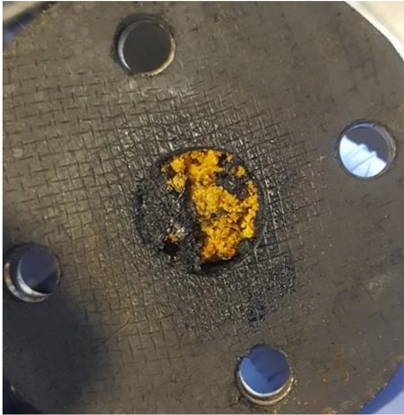
Figure 5.45: PET condensables blockages in pipes at pilot scale
