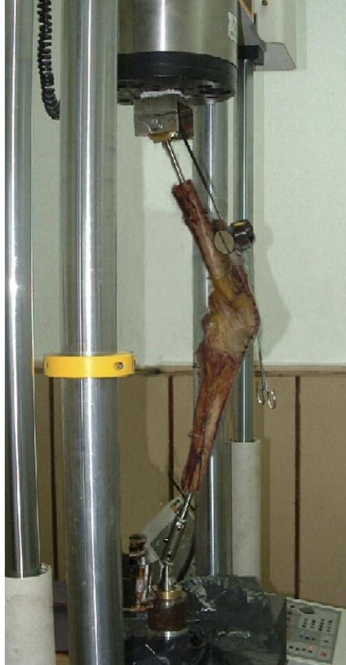
Figure 13: The specimen being tested on a rig exerting 30 kg to the quadriceps muscle (Xu et al., 2007).
