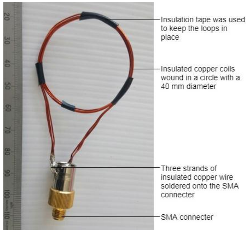
Figure 28: The final antenna design used in the experiments. A ruler is included to show the size in mm.
