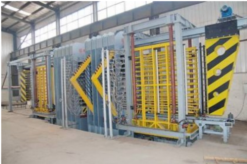
Figure 30: Example of a multi-layered hydraulic WPC hot-press machine to be purchased from Qdguosen (2019)
