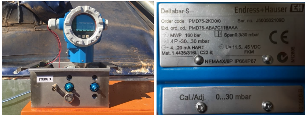
(a) Pressure transducer (b) Specifications (Laubscher, 2017)
