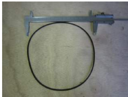
Figure A.11: O-ring ID 160x2 mm
