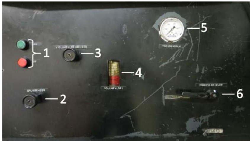
Figure 4.7: Lubrication system control
