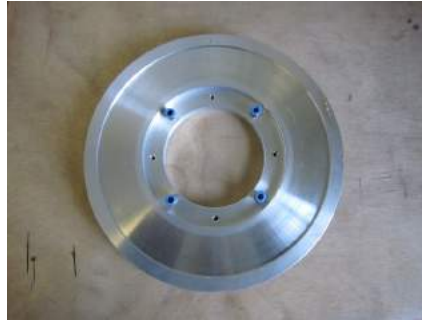
Figure A.10: Rear Diffuser Adapter Plate with Festo pressure fittings
