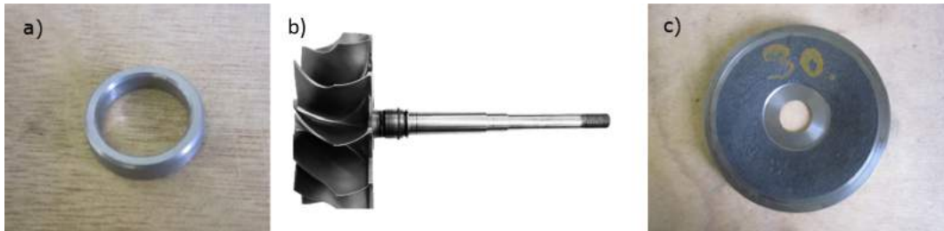
Figure A.15: Turbine spacer (a), Airsearch Turbine shaft (b) and Heat sink (c)
