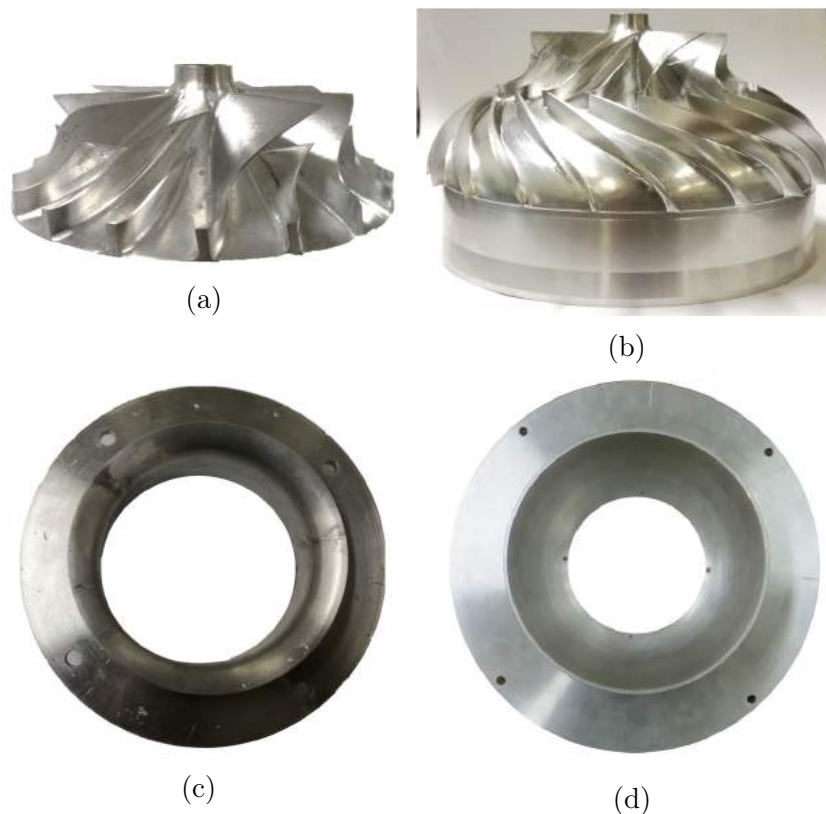
Figure 5.2: Compressor Test Bench Key components: a) Impeller, b) Cross-over Diffuser, c) Impeller Shroud and d) Diffuser shroud
