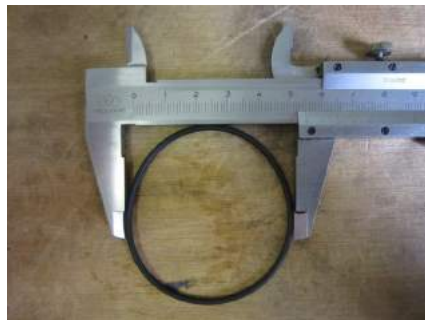
Figure A.8: O-ring ID 55x2 mm
