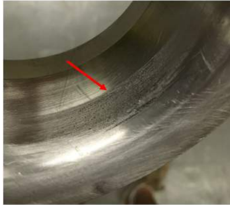
Figure 5.10: Effect of Blade interference on Shroud
