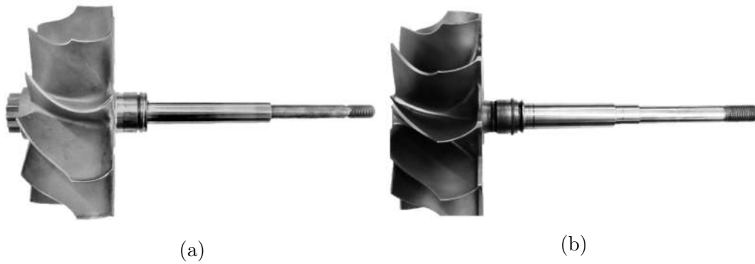
Figure 5.6: Shaft Modification: a) Old Shaft and b) New Shaft
