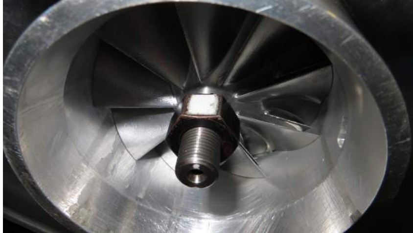
Figure 4.5: Reflector for speed measurement
