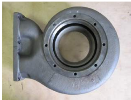
Figure A.19: Airsearch Turbine casing
