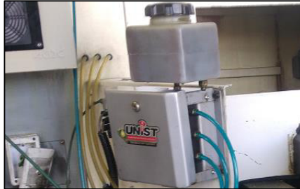
Figure 4: MQL System Implemented in Turning Cell 3
