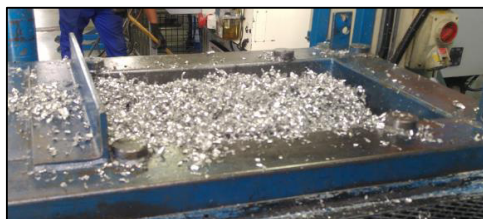
Figure 6: Loose scrap fed into briquetting machine
