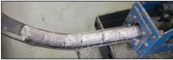
Figure 7: Aluminium briquettes produced
