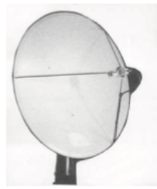
Primary-fed paraboloids. Feed supported by struts (left) and self supported (right)
