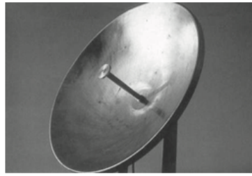
Primary-fed paraboloids. Feed supported by struts (left) and self supported (right)
