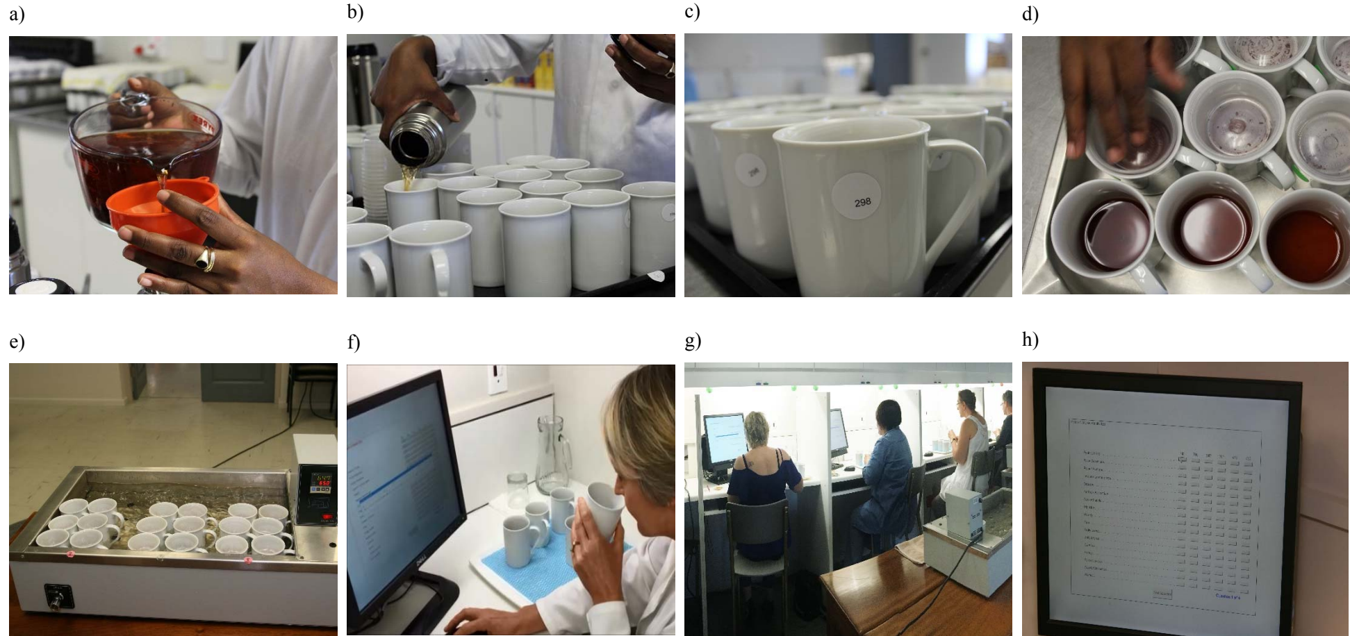
a) Tea (12.5 g), infused in 1 L freshly boiled distilled water for 5 min before straining into preheated stainless steel flasks b) Infusions poured into pre-heated porcelain mugs c) Mugs coded with three-digit random code d) Mugs covered with plastic lids to prevent loss of volatiles e) Mugs presented in random order per assessor in scientific water bath at 65°C to maintain temperature f) Descriptive sensory analysis of infusions using Compusense 5 software g) Samples served in waterbath per assessor h) Score sheet for evaluating full sensory profile of honeybush infusions
