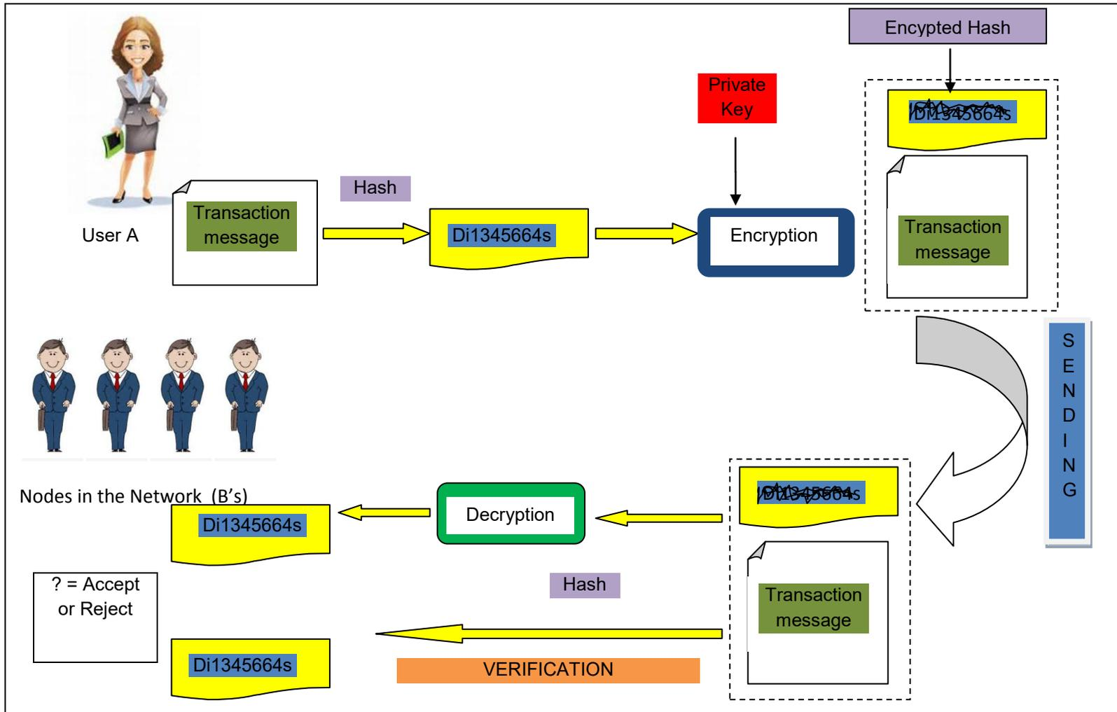
**Figure 4.2 The blockchain digital signature (Asymmetric cryptography)**
