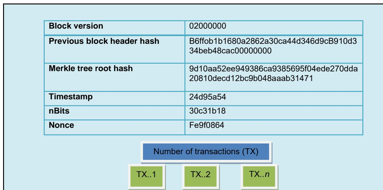
**Figure 4.5** An illustration of the contents of a block
