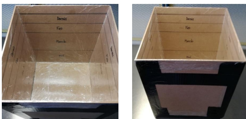
Figure 92: The mould used to cast the 2.4 GHz rhinoceros flank model.
