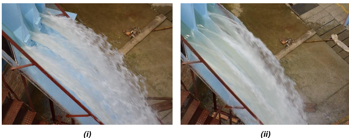
Figure 6.20: Photographs comparing the projected trajectory for the unit discharges of (i) 50 m 2 /s and (ii) 100 m 2 /s.
