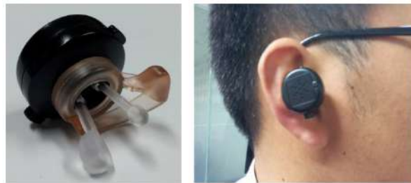
Figure 2.13: Device to measure ear pulse waves due to the cardiac cycle (Park et al. , 2015)
