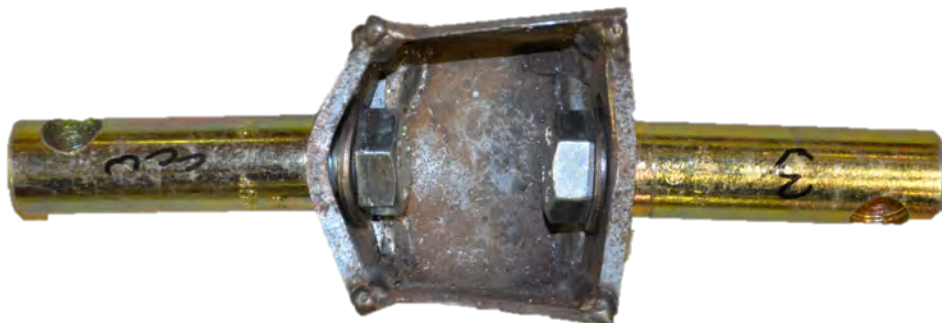
Figure A.2: Shorter vertical connection box after tensile test, l = 50 mm.
