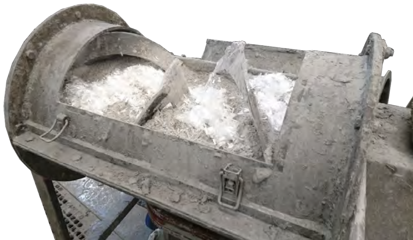
Figure 3.1: Dry ingredients in 70 L paddle mortar mixer
