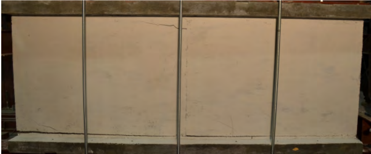
Figure 5.7: PST 1: Fourth nonlinear displacement region, notable lateral slip at the top horizontal connection - indicated by localised cracking.
