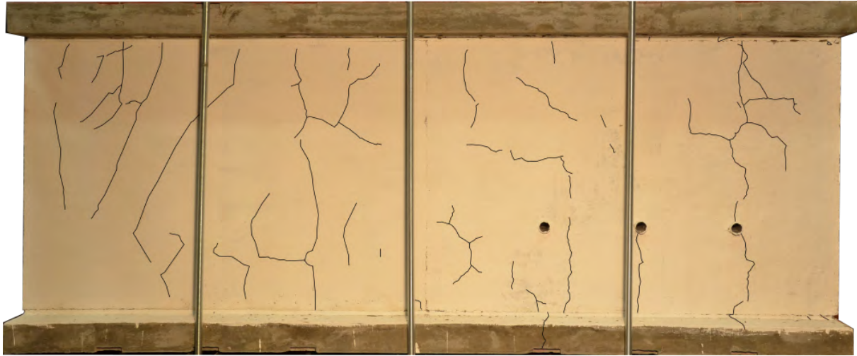
Figure 5.60: Final cracked state for physical test, PST 2
