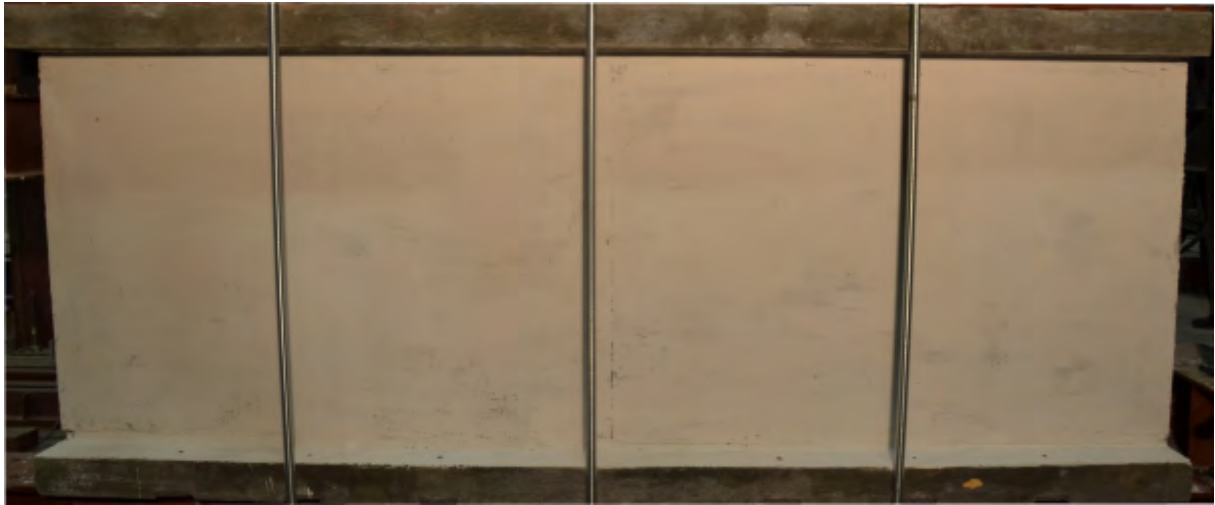
Figure 5.4: PST 1: First nonlinear displacement region, cracking along the lower horizontal connection.
