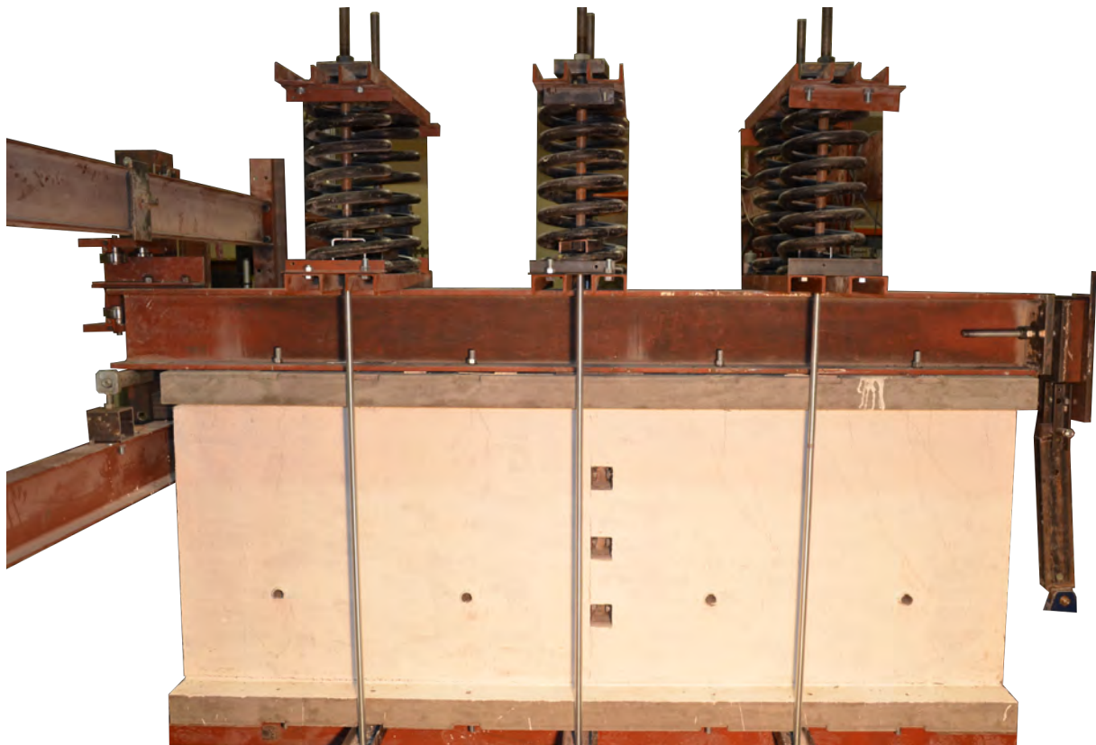
Figure 3.18: Physical scale test laboratory setup for vertical load springs showing the left lateral support frame and pinned vertical support in part
