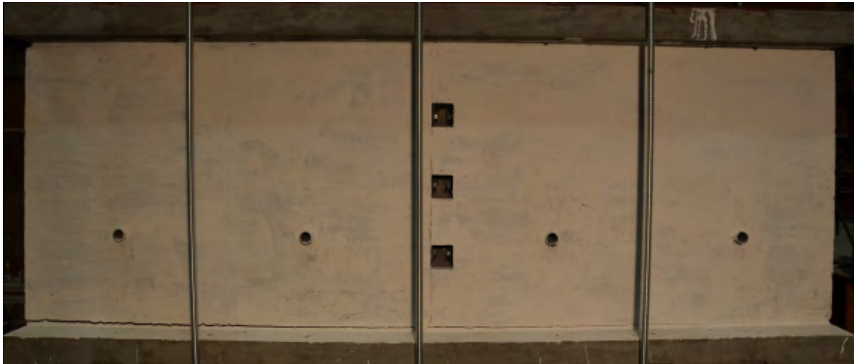
Figure 5.20: PST 3: Second nonlinear displacement region, rotation of connected LWFC panels.
