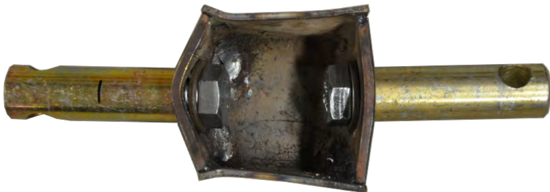
Figure 5.30: Tested connection box showing yielded side at out-of-plane horizontal slot.
