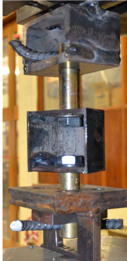
Figure 5.29: Vertical connection box test setup in 250 kN Zwick MTM under tensile load
