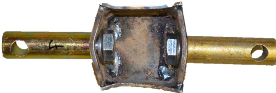
Figure A.1: Longer vertical connection box after tensile test, l = 70 mm.
