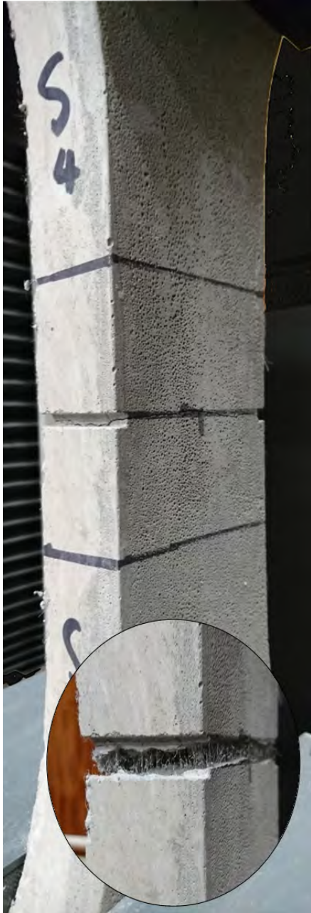
Figure 4.2: Notched dog-bone UTT specimen showing successful tensile crack and visible polypropylene fibres (circled).
