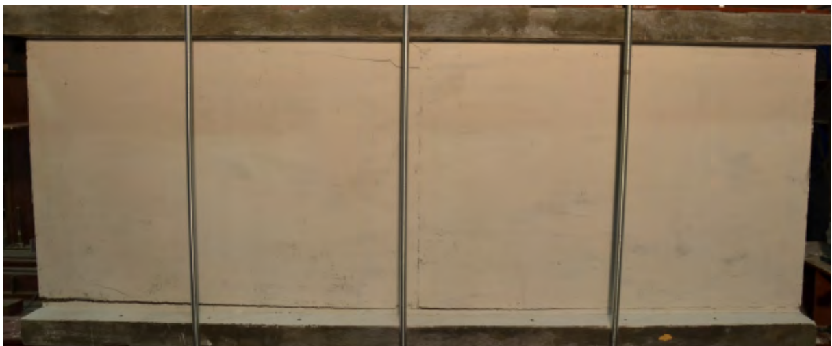
Figure 5.6: PST 1: Third nonlinear displacement region, continued lifting on the LHS and individual panel rotation.
