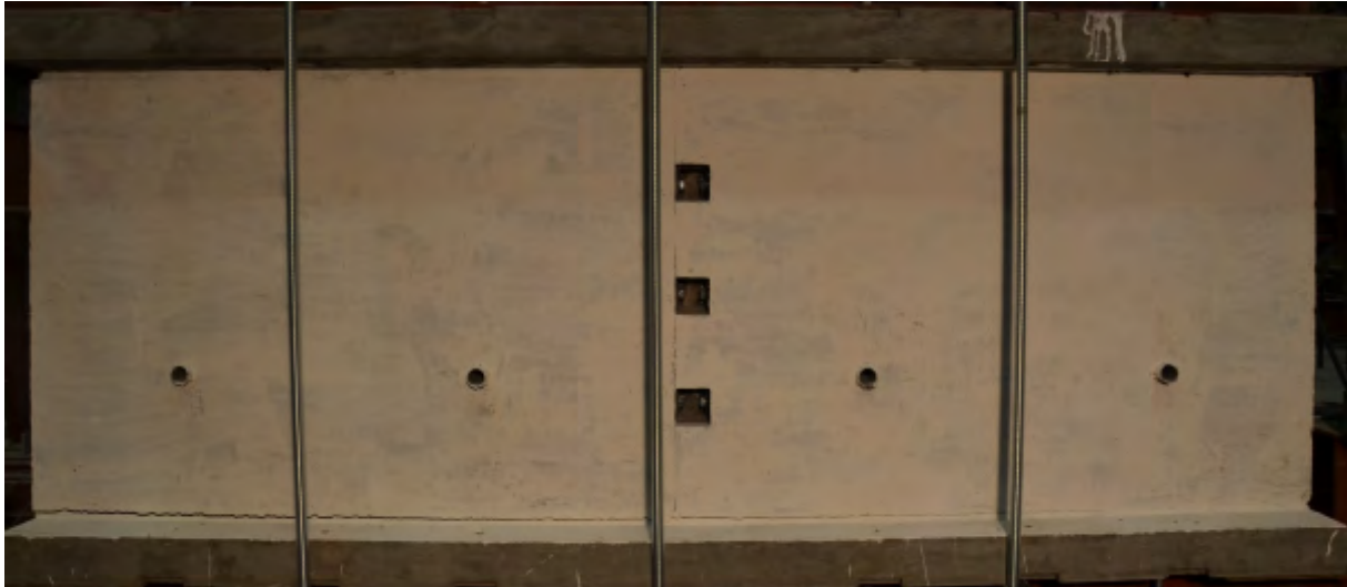
Figure 5.19: PST 3: First nonlinear displacement region, lifting on the LHS and global panel rotation.
