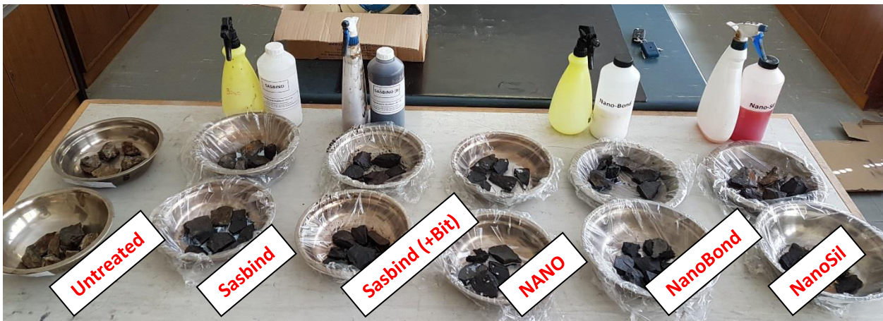
Figure 39 - Sample preparation (or treatment) with DECL liquids prior to commencement of the individual absorption tests.
