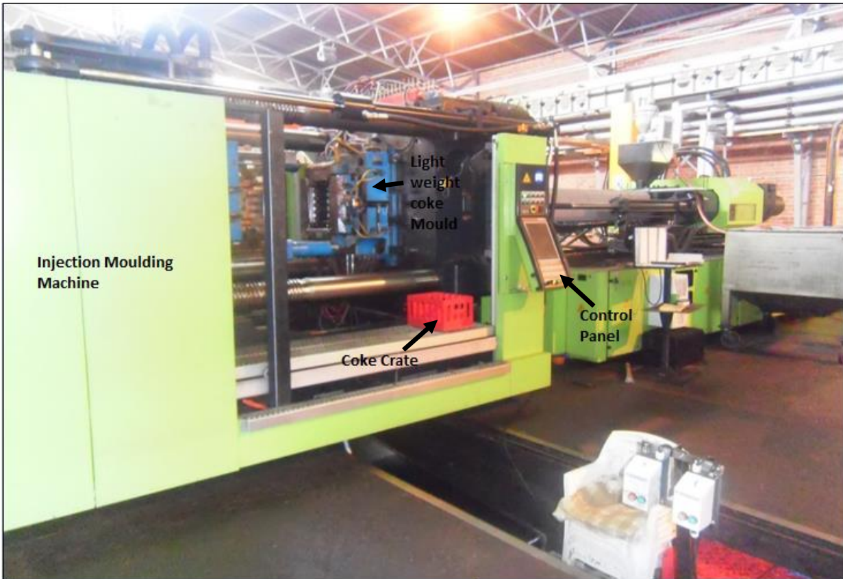
Figure 2: The machine and mould used for the experiments
