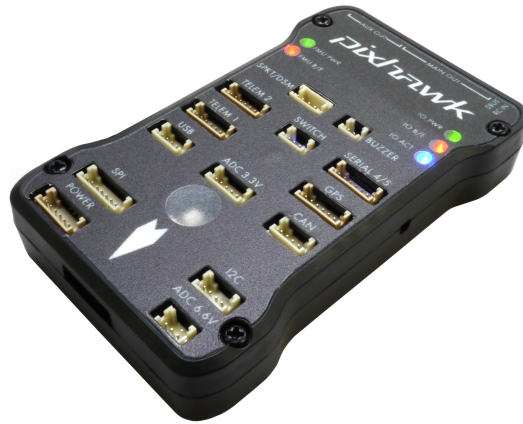
Figure 4.2: Pixhawk flight controller (Pix, 2015).
