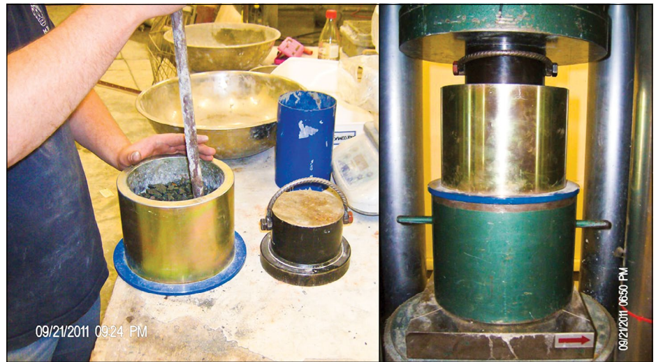
Figure 4 Left: tamping the aggregate lightly, plunger, base plate, steel cylinder and measure Right: assembly in compression testing machine
