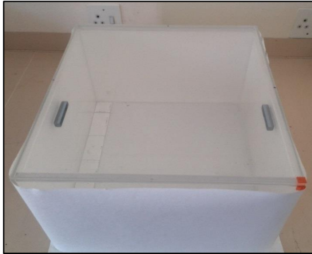
Fig. 3.1. Test arena constructed of Perspex material with all four sides and floor covered with a sheet of white paper.
