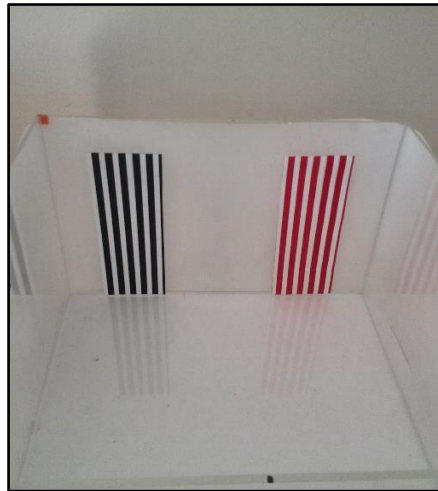
Fig. 3.4. The placement of vertical stripes of black and white, red and white colour patterns and how they were affixed next to each other on one wall inside the arena.
