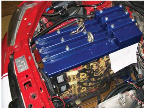
Figure 3.8: Front mounted battery pack.
