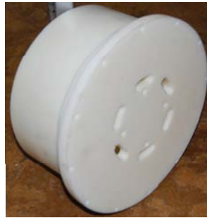
Figure 7.10: Dummy stator for eddy current measurements.
