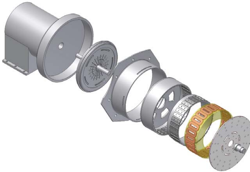
Figure 4.6: Assembly model of the RFAPM machine, clutch and gearbox.
