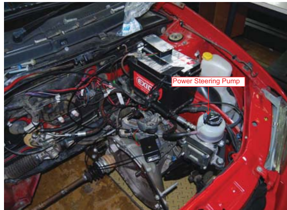
(b) Power steering pump mounted inside the engine bay of the Corsa
