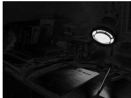
(d) Absolute difference between reference frame and affine adjusted source frame. Note that over-exposed areas could not be corrected.
