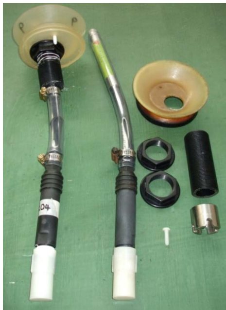
Plate 5.1 Data logger, pH probe and other components of the ruminal pH measuring apparatus.
