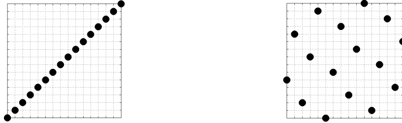
(a) Ill-suited LHD with n_v = 2 and n_p = 16 . (b) Reasonable LHD with n_v = 2 and n_p = 16 .
