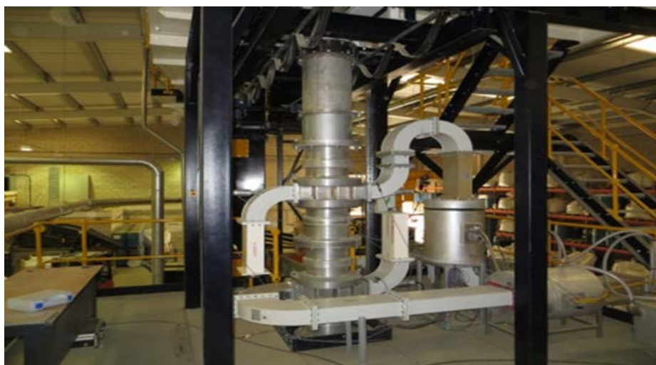
Figure 3. Microwave Applicator Showing 2 Microwave Feeds for the Treatment of Ore at 150 t/hr
