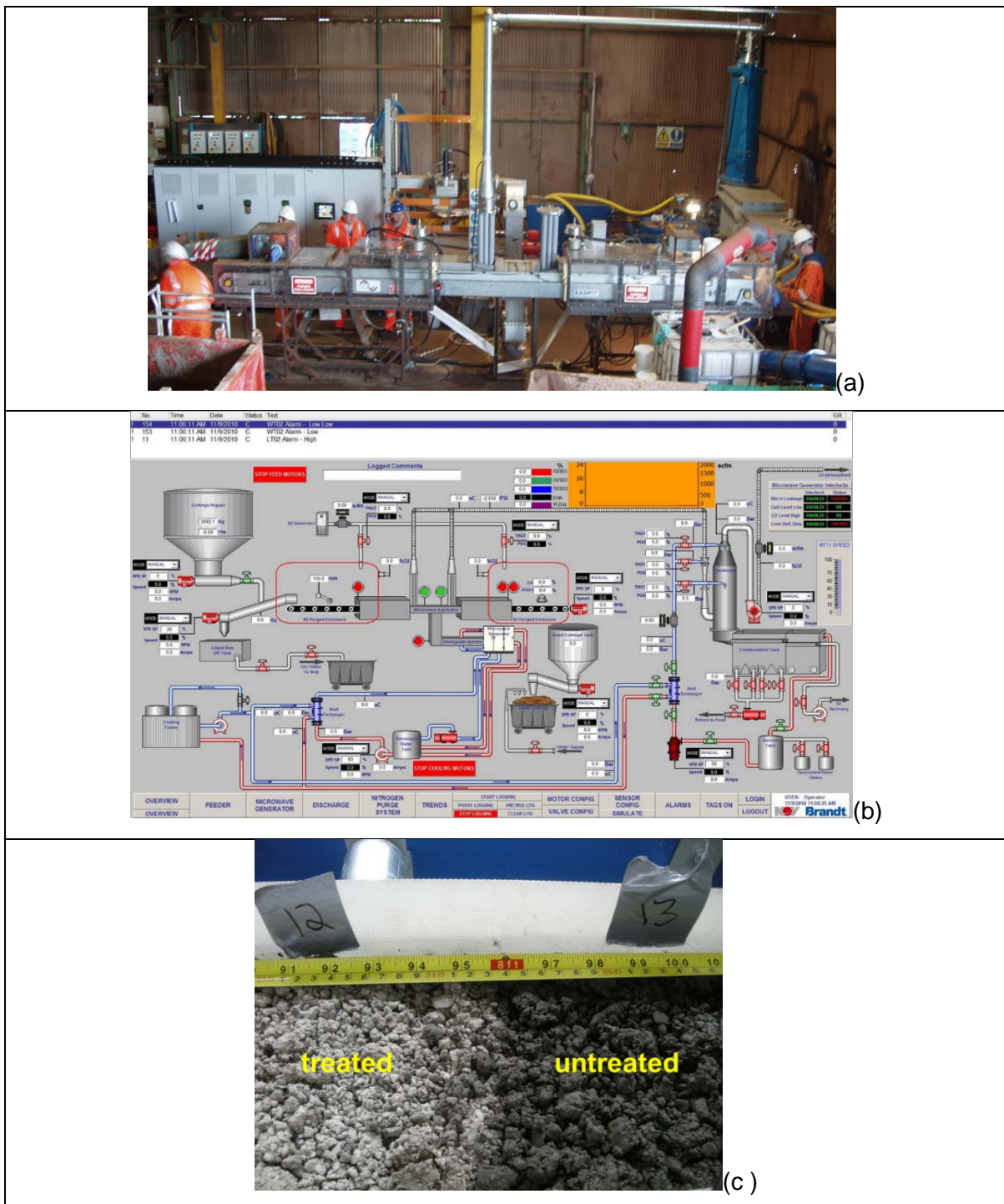
Figure 6 (a) First Industrial Incarnation of Microwave Based System for Processing Oil Contaminated Drilling Wastes, (b), the process control mimic and (c) treated and untreated material.
